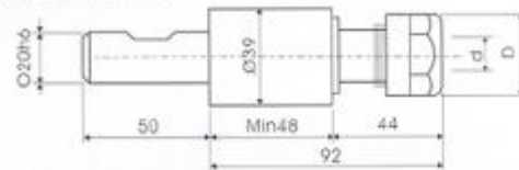
Floating Spindle Adapter (for tapping and reaming application) Patent No.: 79022
